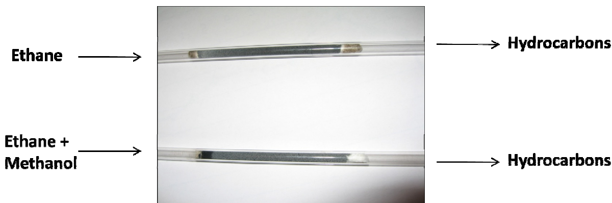
Figure 28: Pictures of catalyst beds from conversion of ethane and co-conversion of ethane and methanol over Ga/H-ZSM-5 at 500 °C after approx. 20 h on stream
