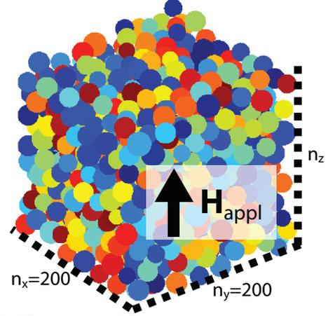
**Figure 1.** [Color online] The powder of packed spherical particles with a normal distribution and with a relative density of the powder sample of 0.52. All spheres have been given a unique color. The aspect ratio of the sample is 1. The dimensions of the sample have been indicated, as well as the direction of the applied field, which is along  $n_z$ .
