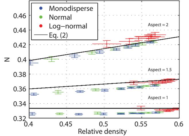
**Figure 2.** [Color online] The demagnetization factor as function of relative density for the monodisperse, normal and log-normal distributions considered, for different aspect ratios. The error bars are the standard deviation calculated for the twenty different samples with the same particle size distribution, aspect ratio and porosity
