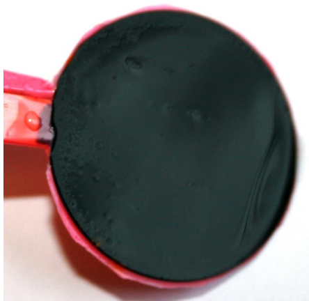
Fig. 36: The as-plated platinum black surface.
