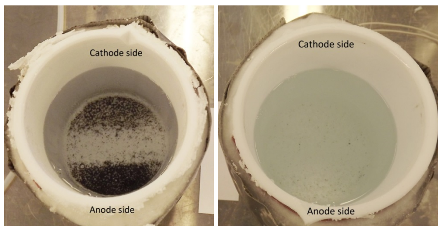
Fig. 63: Left: Black particles found in the electrolyte after over 1600 time of durability testing. Right: the electrolyte in the electrolysis cell after short duration of testing with a new electrolyte.
