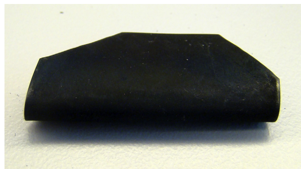
Fig. 11 – Single bend test on a heat-treated and leached PVD Al/Ni 2 electrode.
