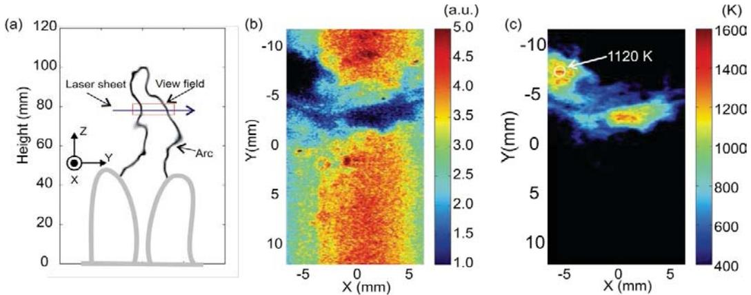
Figure 3: Translational temperature of a gliding arc in horizontal direction at a height of 78 cm; (a) relative position between the gliding arc and the laser sheet (b) Rayleigh scattering signal at 30 ns; (c) temperature image (the average temperature in the labeled circle is about 1100 K).
