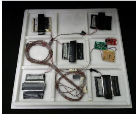
Fig. 5.14. Floor tile without the cover showing the electronics and five cymbals (courtesy of VirginiaTech)
