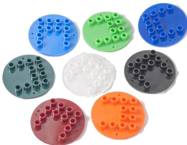
Figure 2.18: Injection moulded chips in different colours. Adding 2% of a master batch to the polymer granulate will fully colour the injection moulded chip.
