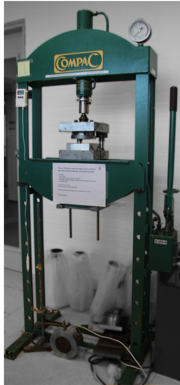
Figure 2.5: Equipment for punching out the nickel shim to the dimensions that makes it mountable in the injection moulder.
