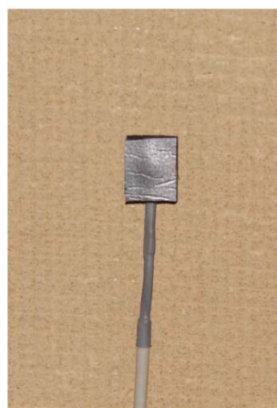
Surface temperature sensor with insulation
