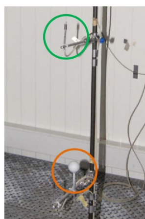
Air temperature sensor Operative temperature sensor
