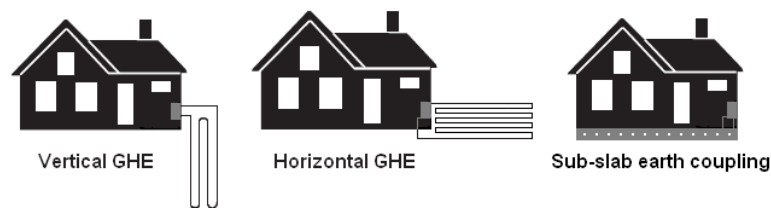
Figure 1. Ground-coupled (closed-loop) systems
