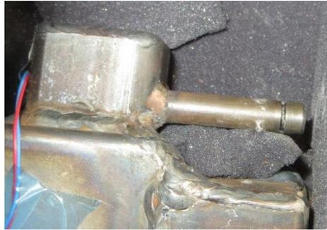
Fig. 4. CO<sub>2</sub> container for activating supercooled sodium acetate water mixture by cooling.
