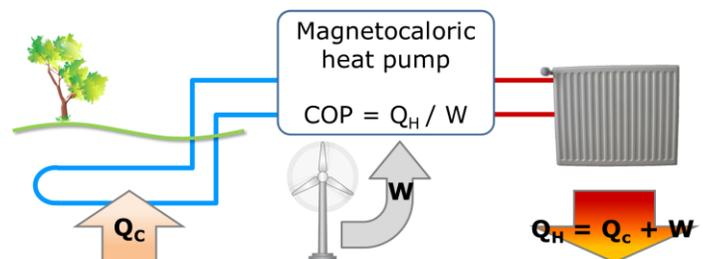
Fig. 2. The magnetocaloric heat pump will move the heat  $Q_c$  from a ground source to radiators or under-floor heating inside a house. The source of the work  $W$  is renewable energy from wind turbines.
