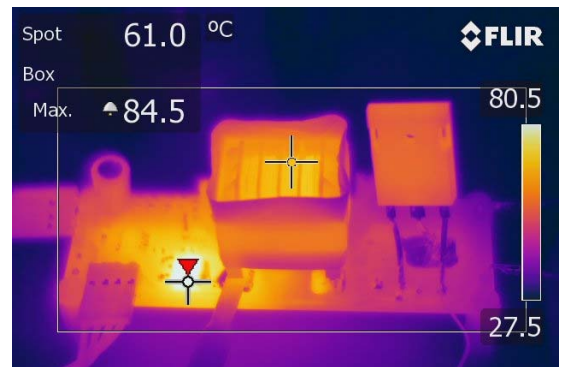
Fig. 9. Steady-state temperature measurement, when the converter is continuously charged and discharged (without any delay between the cycles) from 0 V to 2 kV, and vice versa, when 200 V, 600 m \Omega , 5 A (IRFR220N) low voltage MOSFET is used.
