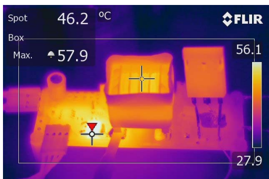
Fig. 10. Steady-state temperature measurement, when the converter is continuously charged and discharged (without 100 ms delay between the cycles) from 0 V to 2 kV, and vice versa, when IRFR220N (200 V, 600 mΩ, 5 A) low voltage MOSFET is used.
