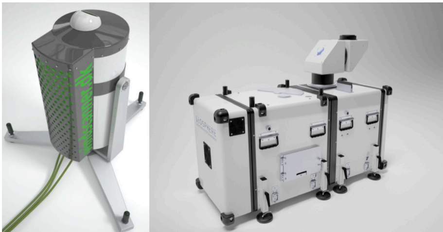
Figure 1.2: The short-range WindScanner (left) and the long-range WindScanner (right)
