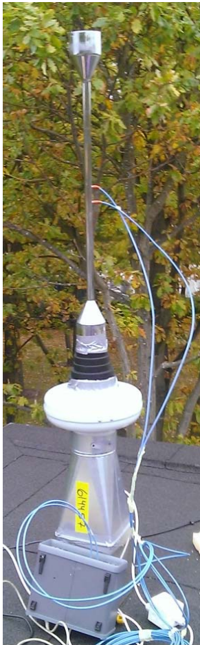
Fig. 7-13 Setup of the experiment to determine the sealing of the roof construction
