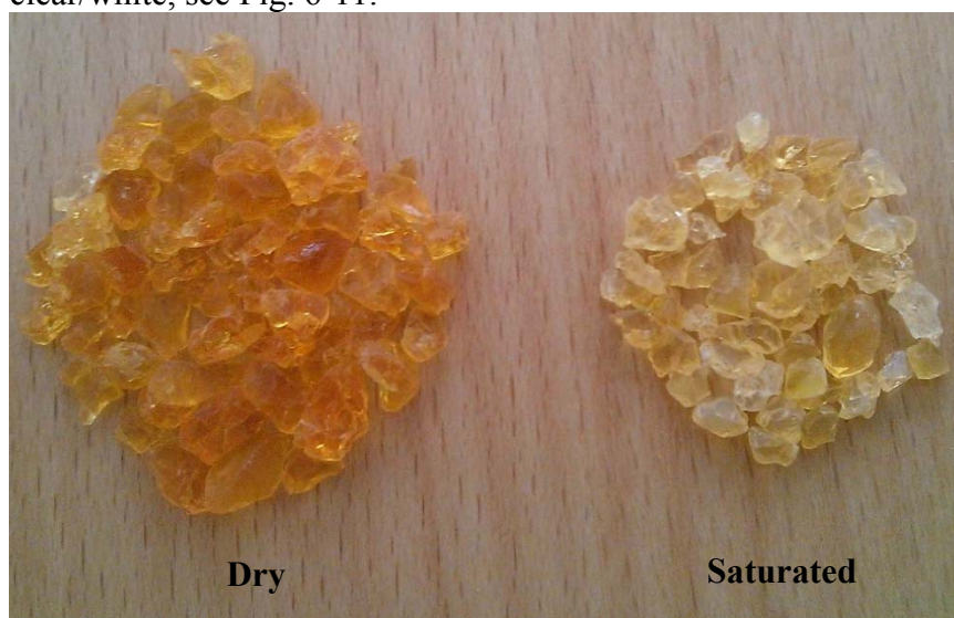
Fig. 6-11 Picture of dry (left) and saturated (right) silica gel
