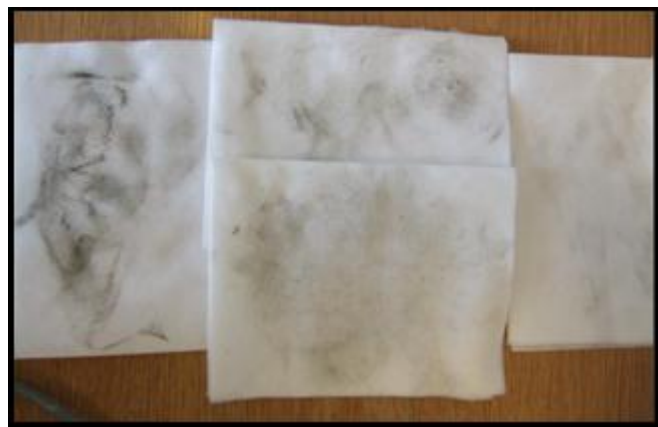
Fig. 7. Showing the amount of dust on the cloths after cleaning the internal glazing surfaces. From left to right shows the cloths used for the glass surfaces number 2, 3, 4 and 5 starting from the outside.
