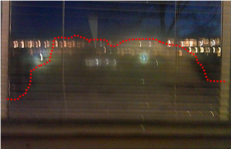
Figure 8 Condensation in the outer cavity for light 2 (K4-100air-K4-50air-K4 in the window
