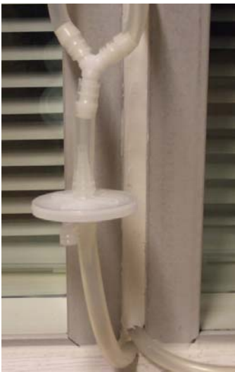
Figure 3 Picture and illustration of the air filter Labodisc 50JP connected to the test window
