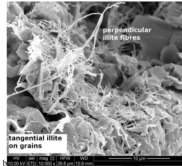
Figure 19: Scanning electron microscopy, SEM, image of illite in a sample from Rotliegend sandstone (Group 3 in Manuscript IV). Both tangential illite on the grain surface and illite fibres perpendicular to grains are observed. [Manuscript IV].
