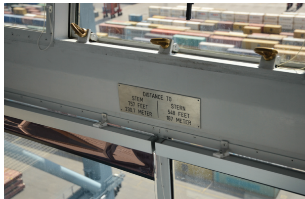
Figure 13.4: Distance from bridge to stem and stern on 15,000 TEU container ship. Photo by Frederik Holten-Tingleff
