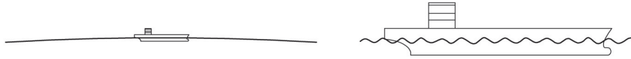
Figure 3.6: Lack of measurable ship response in very low and very high frequency waves. Figure courtesy of Nielsen, 2005.
