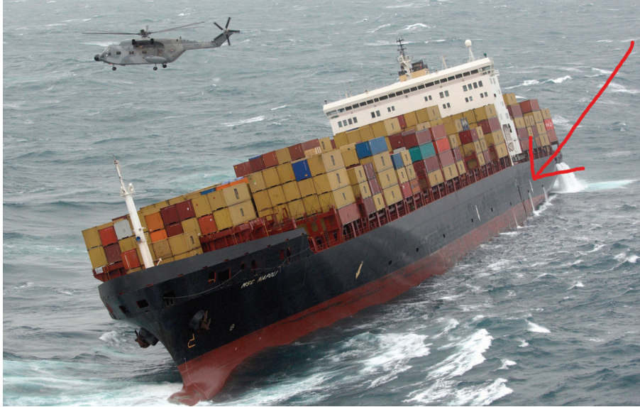
Figure 12.3: 4,420 TEU container ship MSC NAPOLI which broke on 18 January 2007 off the UK coast. Photo courtesy of the French Ministry of Defence.
