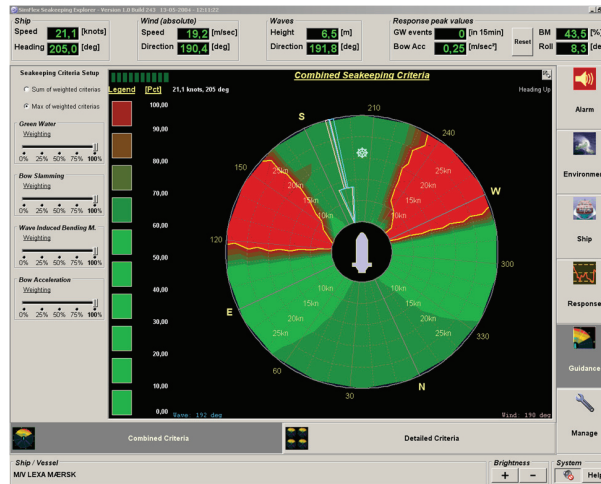
Figure 13.2: Screenshot from the decision support system SeaSense illustrating combined sea keeping criteria in a polar diagram to enable assessment of the navigable combinations of speed and heading.
