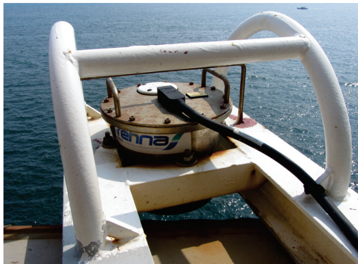
Figure B.6: Port side Radac sensor on board the 9,400 TEU ship. Photo by the author.
