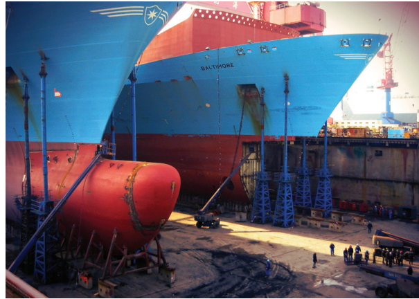
Figure 13.5: Retrofit of new bulbous bows on the Maersk Boston class in 2012. Photo by Maersk Line.
