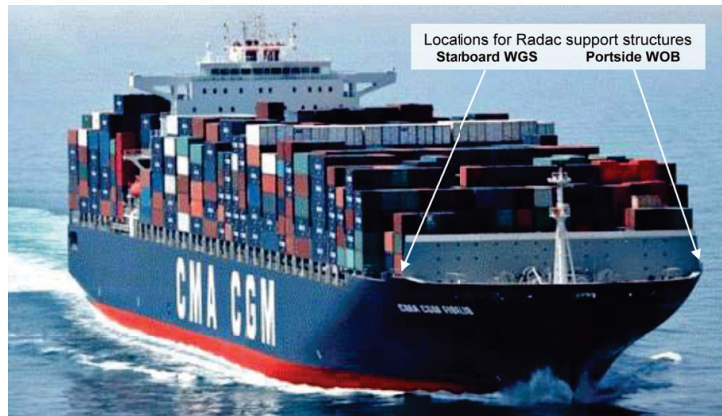
Figure B.5: Location of the two Radac sensors on board the 9,400 TEU ship. Illustration from Fresser (2011)
