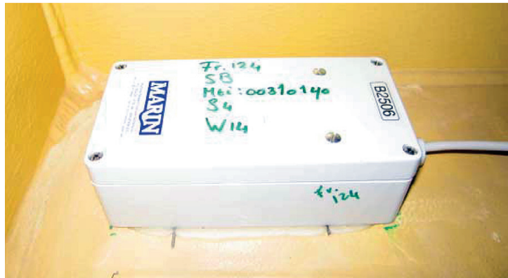
Figure B.7: Acceleration sensor at frame 124 on board the 9,400 TEU ship. Illustration courtesy of MARIN.
