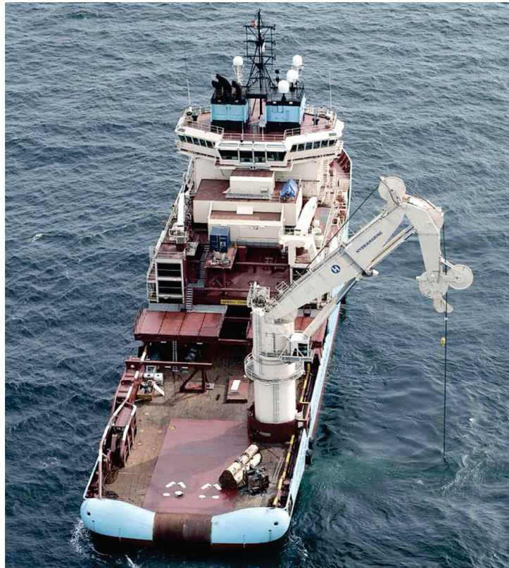
Figure 4.13: Subsea support vessel with heave compensated crane. Photo by Maersk Supply Service.
