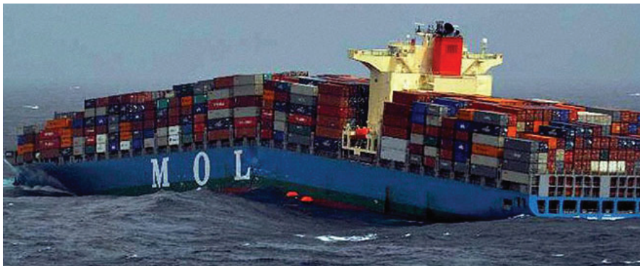
Figure 12.4: 8,540 TEU container ship MOL COMFORT before the vessel broke in two and sank on 17 June 2013. Photo courtesy of PTI Photo.
