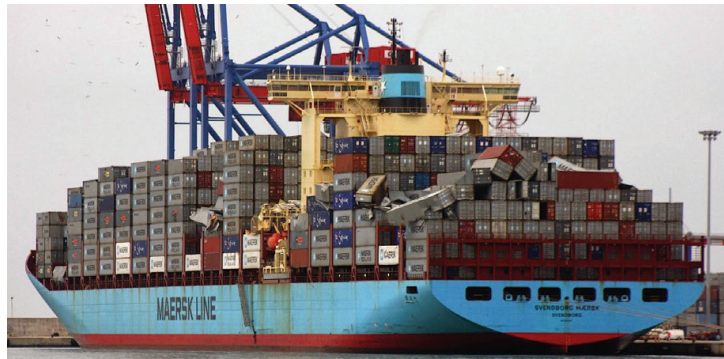
Figure 13.1: 8,600 TEU container ship SVENDBORG MÆRSK after losing over 500 containers over board in February 2014. Photo by Santiago Sáez.
