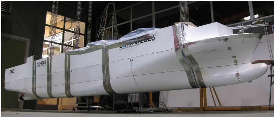
Figure 2.6: Flexible ship model at CEHIPAR. Photo by Camille Fresser.
