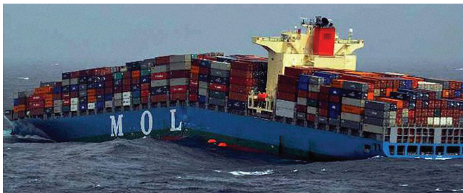
Figure 12.4: 8,540 TEU container ship MOL COMFORT before the vessel broke in two and sank on 17 June 2013. Photo courtesy of PTI Photo.
