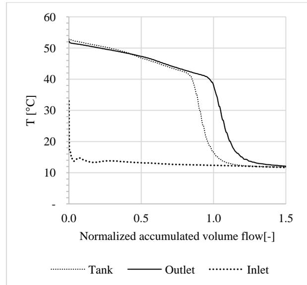
Figure 12: Temperature progress during discharging, measured at inlet, outlet and inside the tank at a height of  $\frac{3}{4}$  of the total tank height.
