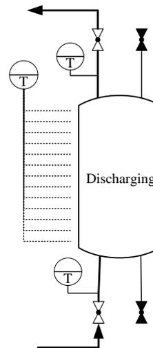
Figure 10: Experimental setup – Discharging the tank
