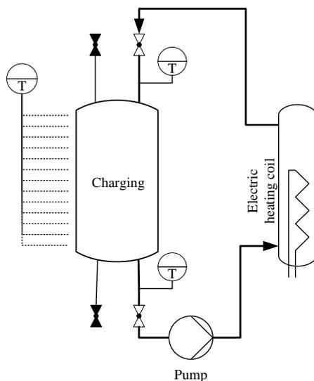
Figure 9: Experimental setup – Charging the tank
