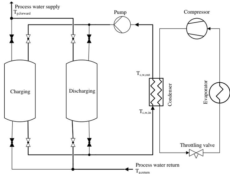
Figure 2: A principle sketch of the ISEC system. One tank is charging, while the other tank is discharging.
