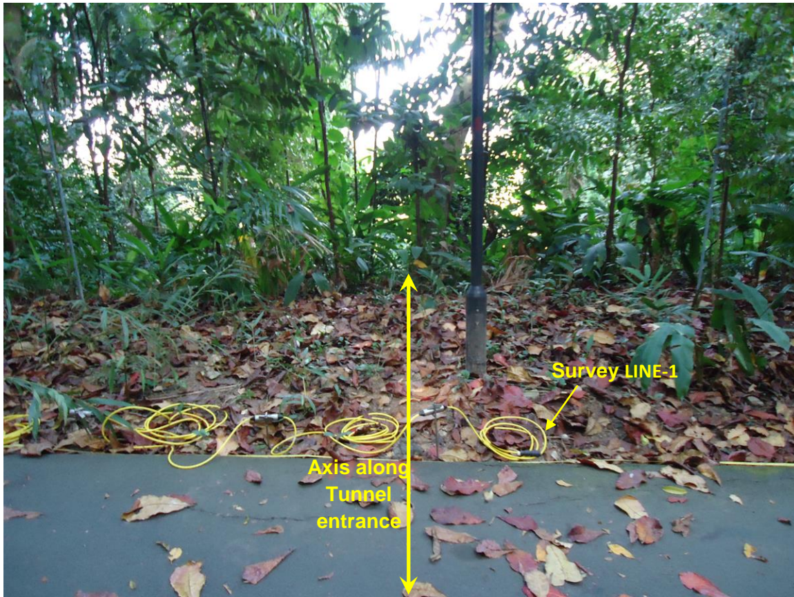
Figure 5-4 Picture showing setup of survey LINE-1 for the geophysical measurement relative to the tunnel axis
