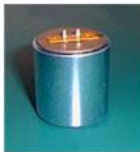
Figure 1-3 Picture of a GS11D vertical component geophone.
