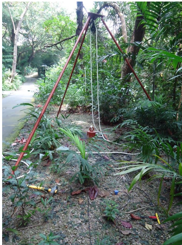
Figure 2-8 Seismic source (weight drop) used in the geophysical survey
