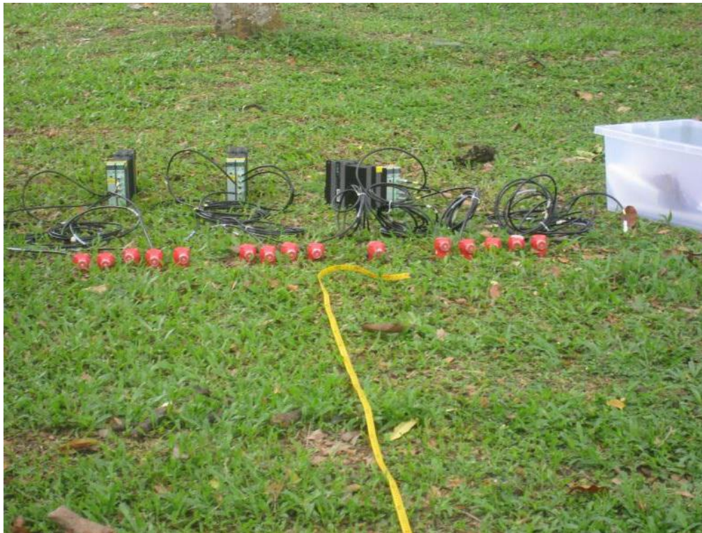
Figure 1-2 Picture of an array of GS11D vertical component geophone array set up on the ground surface for the measurement
