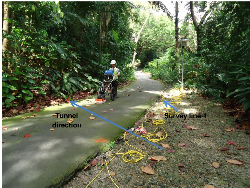
Figure 2-9 Setup of survey line 1 for the geophysical measurement
