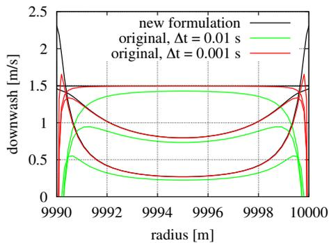
**Figure 6.** Buildup of induced velocities at the elliptical wing with a prescribed circulation at  $t=0.01$  s,  $t=0.05$  s and  $t=5.0$  s, corresponding to 35 cm, 1.75 m and 175 m long trailed wakes. The new formulation, Equation (10), leads to the same results, independent of the time step.
