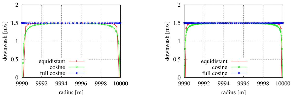
**Figure 5.** Comparison of the steady downwash at an elliptical wing with a wake of 175 m length. The calculation points and vortex trailing points have been distributed using the distribution methods described in Section 2.4. The blade has been discretized using 40 (left plots) or 80 (right plots) calculation points.
