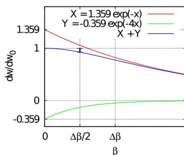
**Figure 2.** Illustration of the exponential trailing functions. The black mark indicates the underestimation of the induction due to the multiplication of  $D_w$  by the exponential factors in Equation (5) for an element with length  $\Delta\beta$ .
