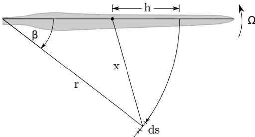
**Figure 1.** Geometry at a blade rotating with the constant angular velocity  $\Omega$ . The downwash at a distance  $h$  from the vortex trailing point shall be computed. Since the infinitesimal vortex element with length  $ds$  has left the lifting line, the blade has been rotated by the angle  $\beta$ .
