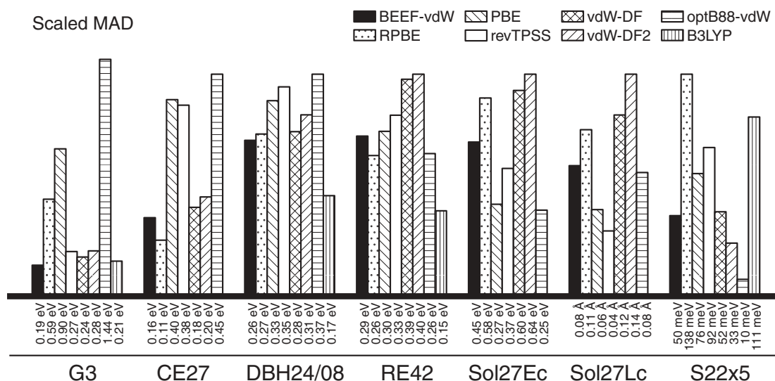
FIG. 9. Bar plot comparison of the accuracy of different density functionals in predicting various materials properties. For each data set, the bars illustrate proportionally scaled mean absolute deviations. The data sets are chosen to represent intramolecular bond energetics (G3), chemisorption energetics of molecules on surfaces (CE27), molecular reaction barrier heights (DBH24/08), molecular reaction energies (RE42), bulk solid cohesive energies (Sol27Ec) and lattice constants (Sol27Lc), and interaction energies of noncovalently bonded complexes (S22x5). B3LYP calculations were not performed for bulk solids nor the extended CE27 systems.
