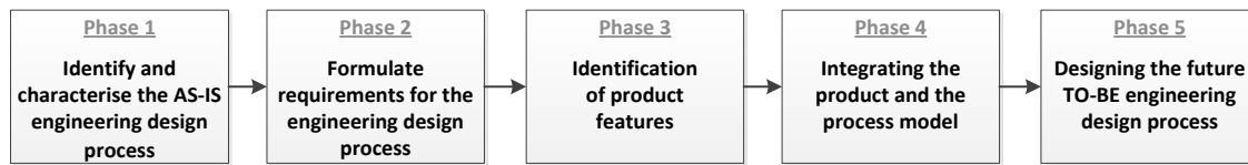
Figure 1: Phases for Developing Engineering Design Processes
