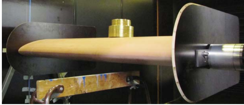
Figure 3.8: Photo of static test. 20 kg additional weight was placed on the airfoil.
