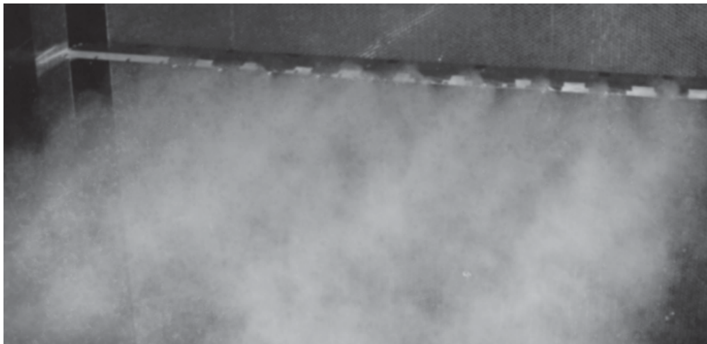
Figure 3.2: Spray system produces cloud in the wind tunnel. The system includes 15 evenly spaced nozzles.
