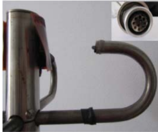
(b) Photo of one of the arms and the connector of HoloOptics ice rate sensor in summer 2012.
