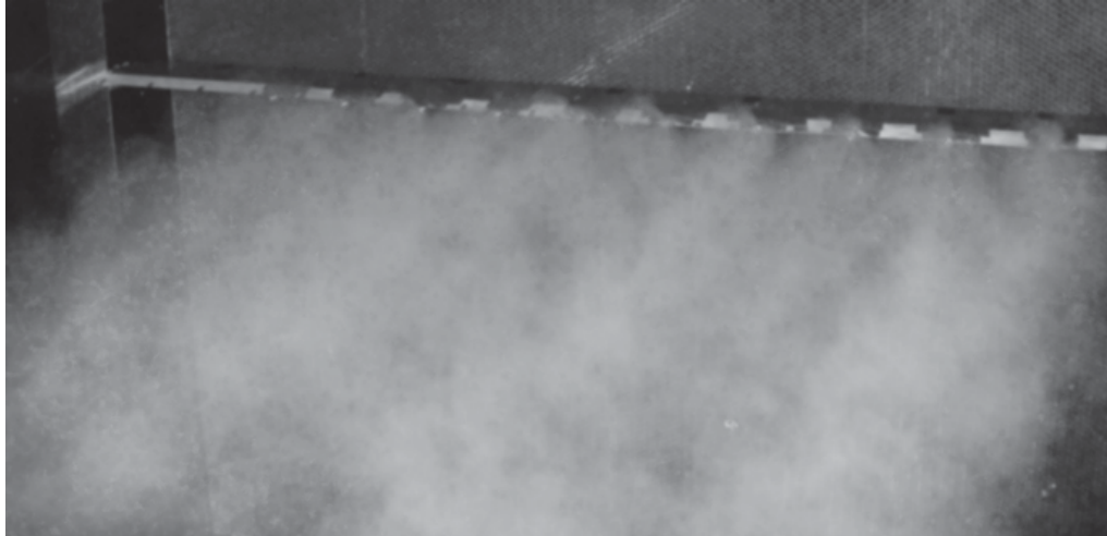
Figure 3.2: Spray system produces cloud in the wind tunnel. The system includes 15 evenly spaced nozzles.
