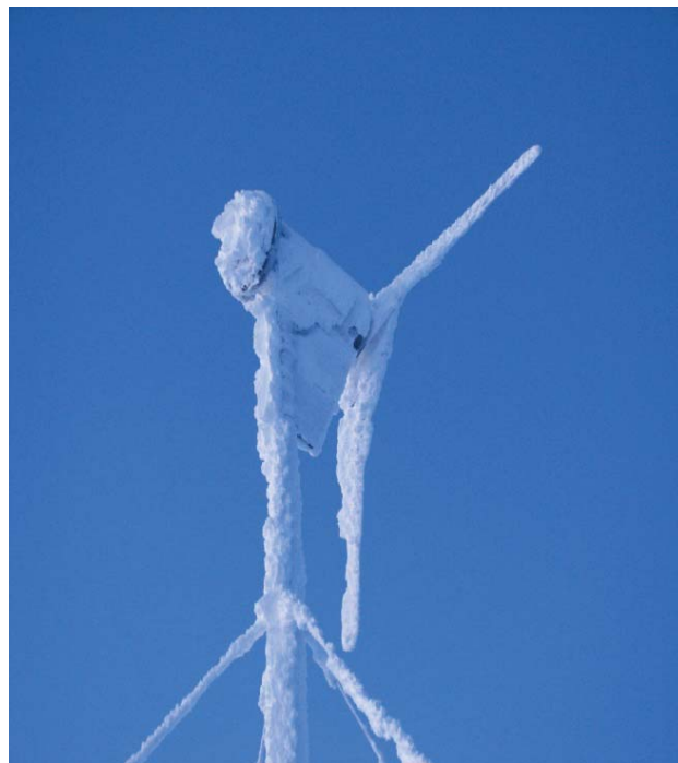
Figure 2.1: Iced 6kW Proven turbine at Summit Station, in Greenland. This level of icing reduces power output by 80 % or greater. (Dahl [2009])
