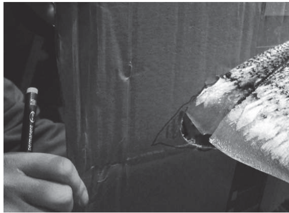
Figure 5. Example for ice layer contour tracing.
