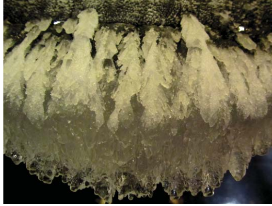
Figure 3.22: Photo of the 4^\circ angle of attack mix ice test in case of Re \simeq 1E6 , MVD \simeq 25\mu m and LWC \simeq 0.65g/m^3 for a NACA 64-618 profile.
