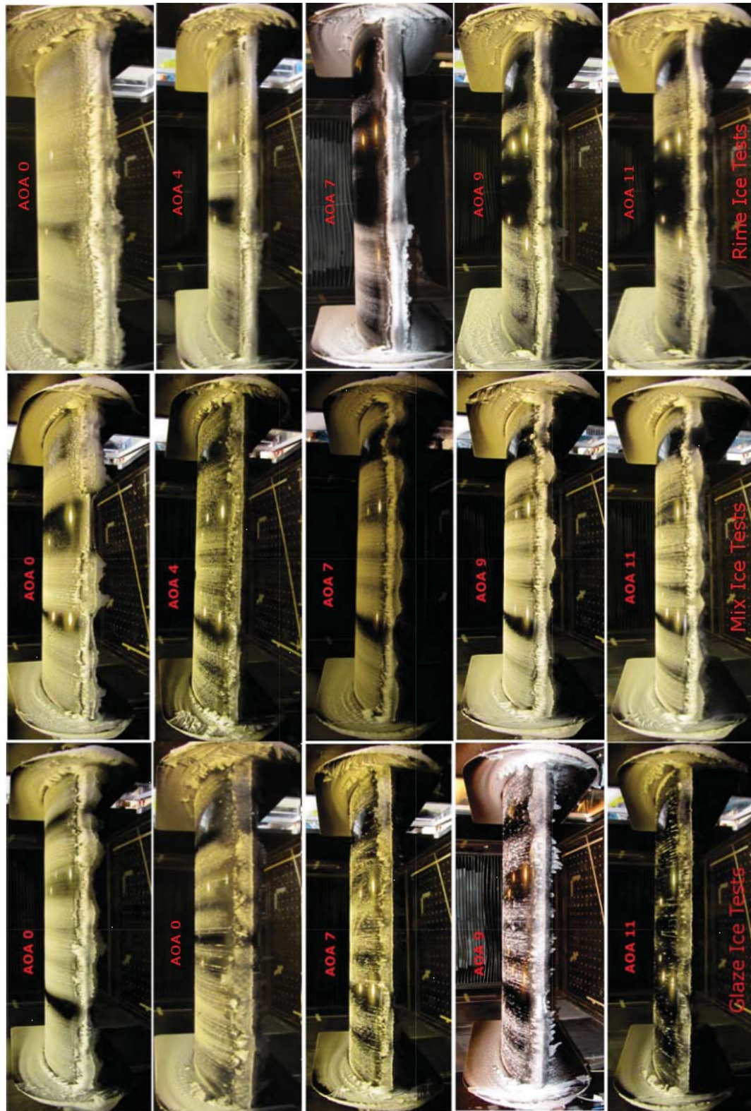
Figure 3.13: Iced blade profiles at the end of the accretion tests for the different types of ice at each angles of attack.
