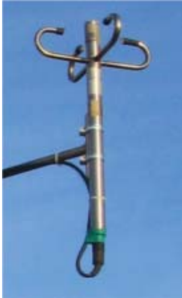
(a) Photo of the HoloOptics ice rate sensor after installation in summer 2011.
