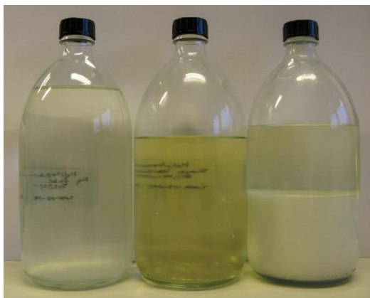
Figure 6.5: The collected fractions of product streams from the setup during continuous operation. To the left is the aqueous waste from the decanter, at the center is the organic phase containing dehydrated product 5 and to the right is the crystalline melitracen HCl 6 API and the mother liquid.
