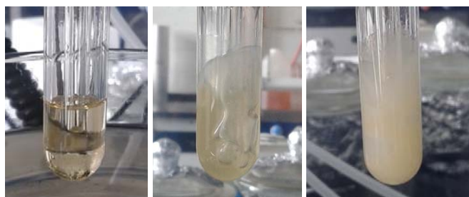
Figure 8. Absorption stages in dry [N6666][Pro]. The IL is initially transparent (left) but a turbid phase appeared during absorption (right).
