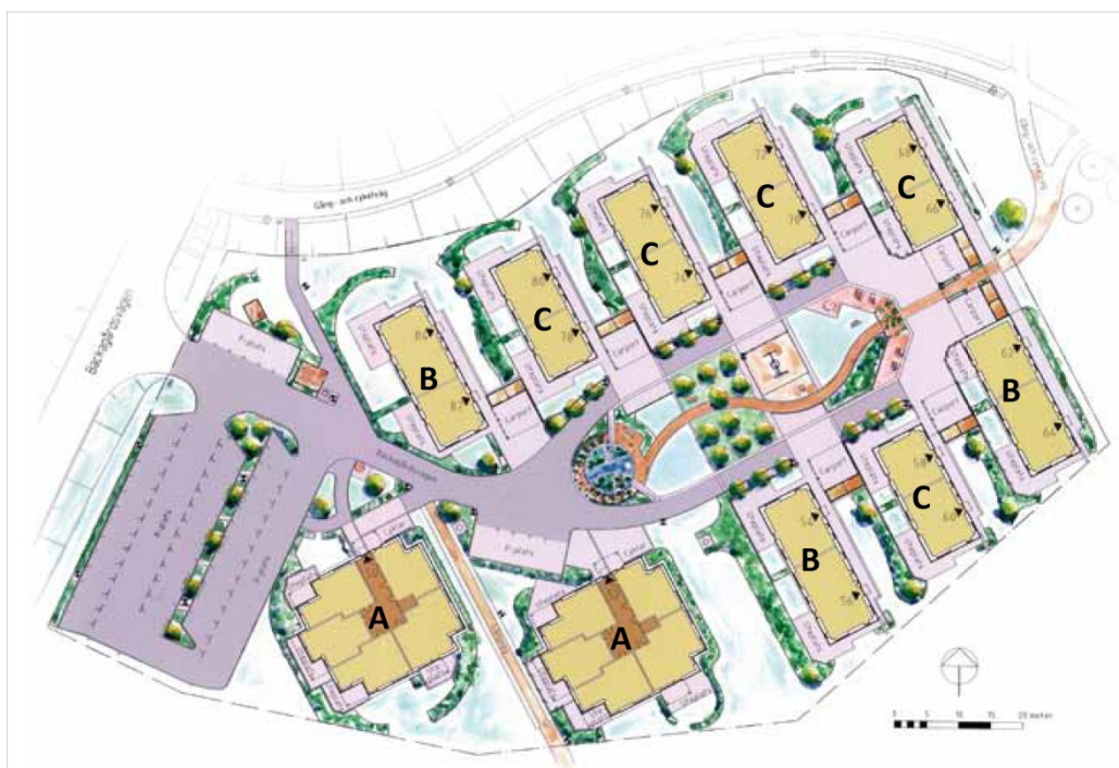
Figure 2. Principal site plan of the Söndrums Kyrkby multi-family and pair passive house ground site. Building types are: (A) Multi-family houses, (B) Pair-houses with a two-room and a four-room apartment, and (C) Pair-houses with two three-room apartments. Source: [3].
