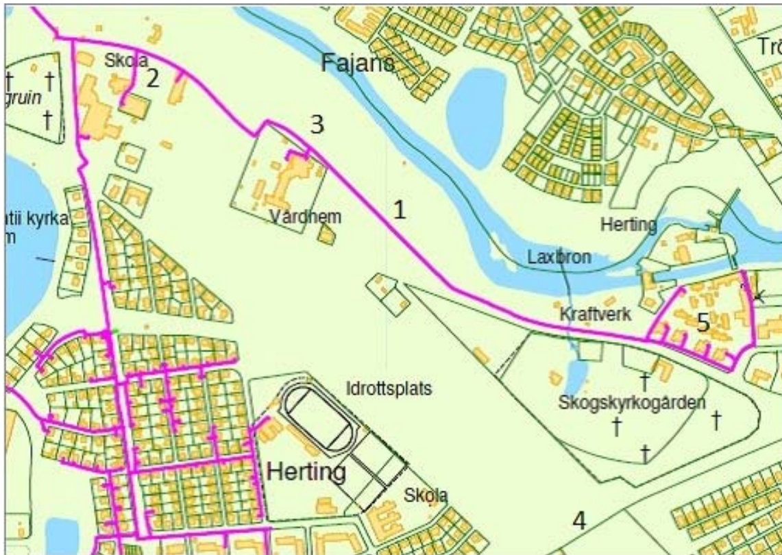
Figure 9. Overview of heat distribution pipe line to Hertings gård from Falkenberg city district heating network. Source: [16].
