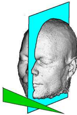
Figure 12: Spin is influenced selectively in a sagittal slice, if a gradient from left to right is applied while radio waves are transmitted.
