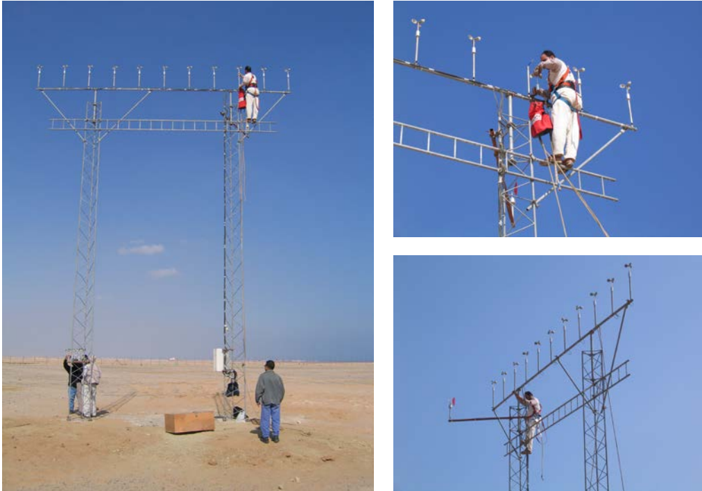
Figure 1. Cup anemometer calibration facility at Hurghada WETC: upwind fetch to the NW (left) and details of the cup anemometer set-up (right).
