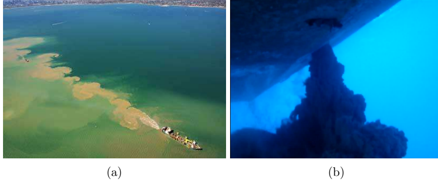
FIG. 1: a) Overflow turbidity plume , b) Dredged material disposal
