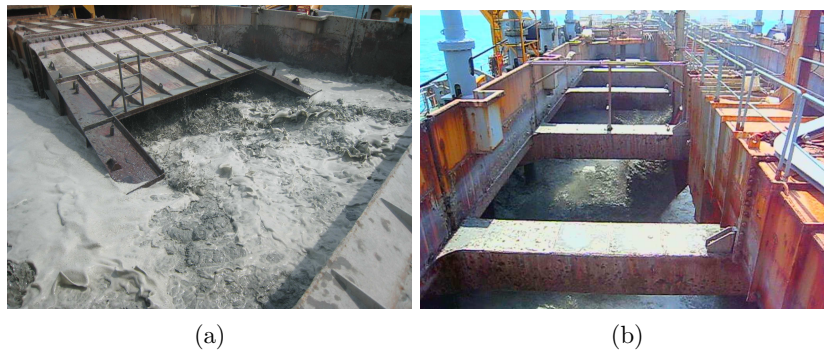
FIG. 5: Inlet configuration , a) Main inlet , b) One of the secondary inlets
