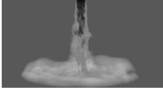
FIG. 1: 3D view of the volumetric concentration contours, \epsilon = 0 and F_d = 2.2 . The contours have threshold of 300\text{mg/L} .
