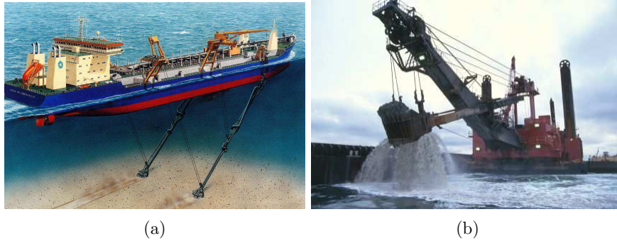
FIG. 2: a) Trailing Suction Hopper Dredger (TSHD) , b) Mechanical Dredger
