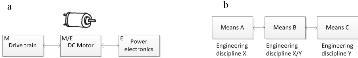
Fig. 14 (a) The dc motor has stakeholders within mechanical and electronics engineering discipline. (b) The generic aspect of the ‘Multi-disciplinary means dependency’
