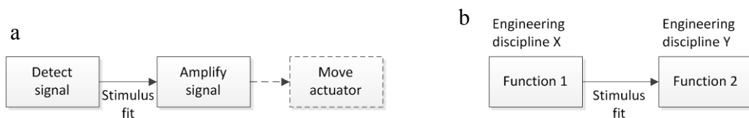
Fig 8 Example of how the amplifying function responds to the input (a). The generic aspect of the ‘response function dependency’(b)
