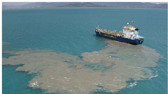
Figure 2.14 Dredged material ready to dumped from a split hopper, Right: The sediment plume due to dispersion and mixing of fine material after dumping
