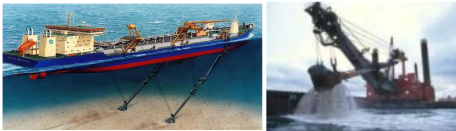
Figure 2.3 Trailing suction hopper dredger, Right: Mechanical Dredger
