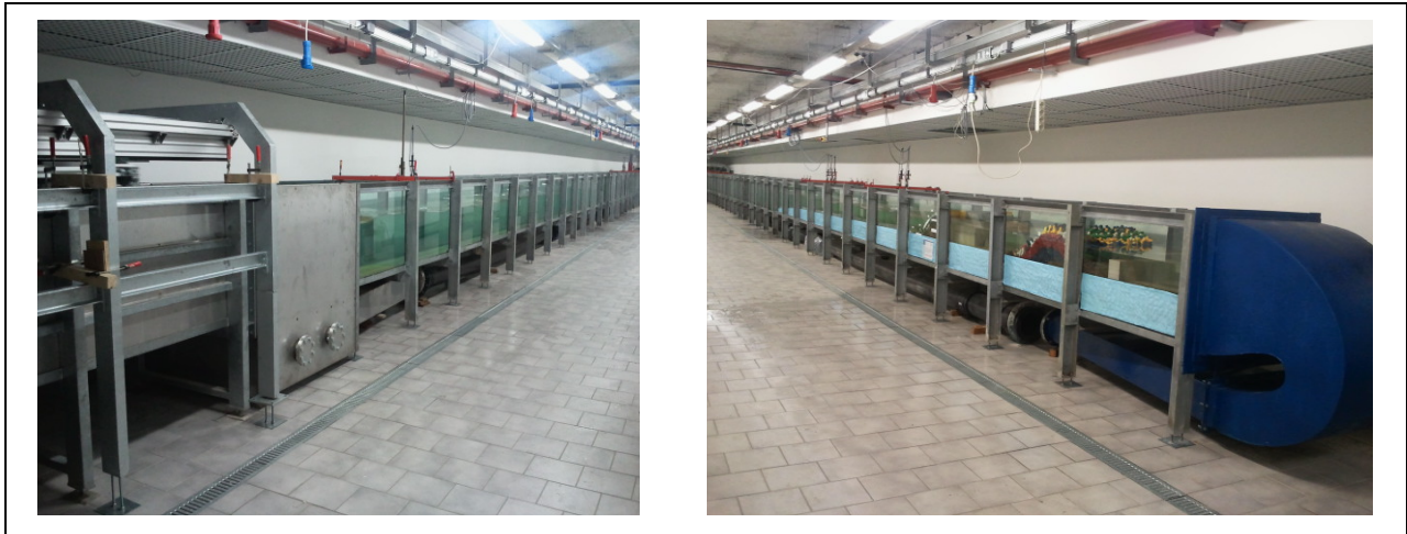
Figure 4.1 COAST-Lab wave-current flume of Florence University.
