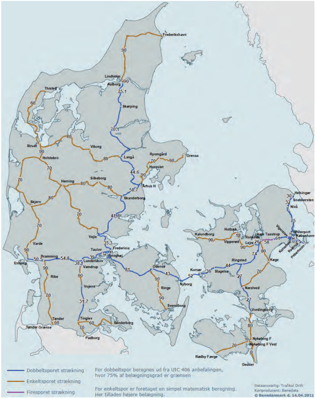
Figure 9.7: Peak hour capacity consumption in percent [%] of railway line sections for the yearly timetable in 2010. Double track lines are marked with blue, single track lines with brown and quadruple track lines with purple. Recommended maximum capacity consumption is 75% for double track lines (RND 2011b)
