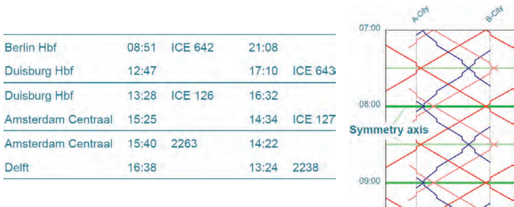
Figure 4.8: Example for a symmetric periodic timetable – public timetable for train service (left) and schematic graphical timetable (right) (Liebchen 2006)
