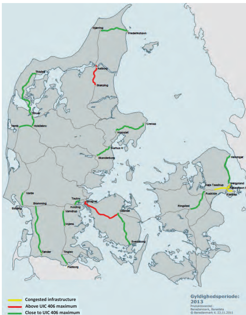
Figure 6.15: Overview of capacity bottlenecks and officially declared congested infrastructure in the Network Statement 2013 by Rail Net Denmark (RND 2012a)
