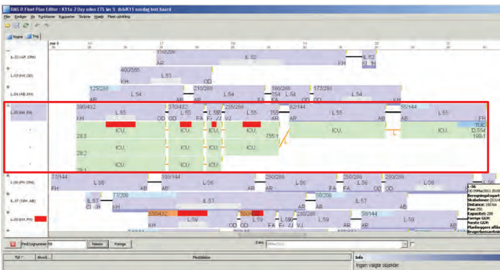
Figure 3.13: Screenshot from DSB's OMPLS2 software tool for preparing rolling stock rostering plans (Madsen 2010)
