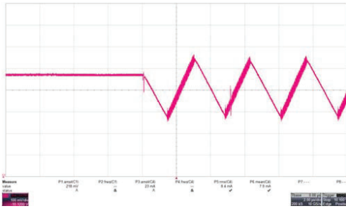
(a) v_{out}(t) : 200 mV/div, 5 \mu s/div. Load step from 0 to 0.5 A.
