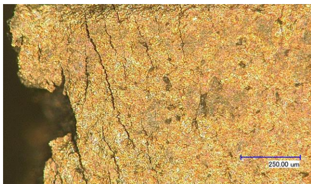
Fig.1. Brittle fracture of the layer on the fatigue scrap
