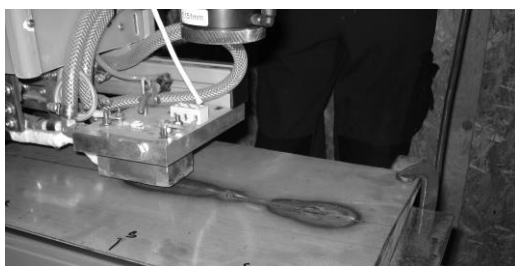
Fig. 2. Production of weld on a massive steel plate
