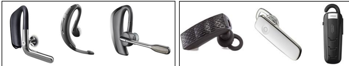
Figure 5-3 The groups of behind - the - ear and in - the - ear bluetooth headsets
