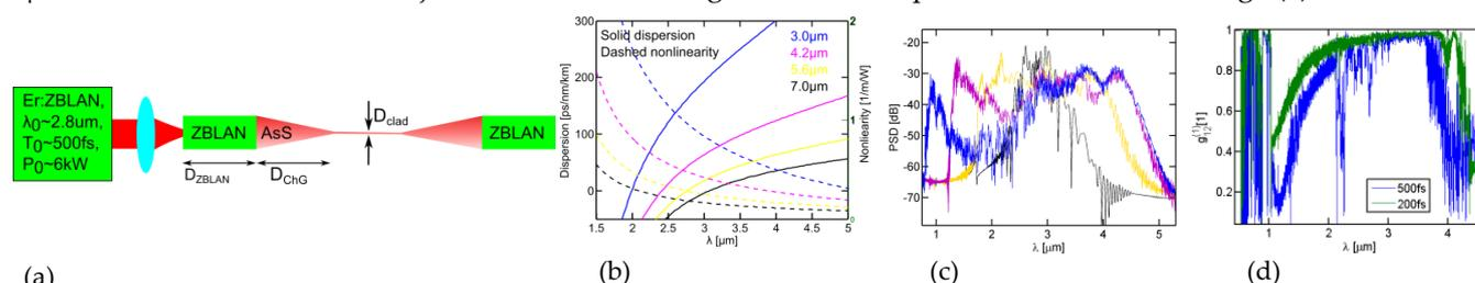
(a) Mid-infrared supercontinuum setup with a 2.8 $\mu$ m mode-locked laser, collimating lens and fluoride-chalc fibre taper. (b) Dispersion and nonlinearity at the taper waist for different cladding diameter. (c) Simulated supercontinuum. (d) Coherence for 200 and 500fs pulses durations supercontinuum in the 3 $\mu$ m taper.
