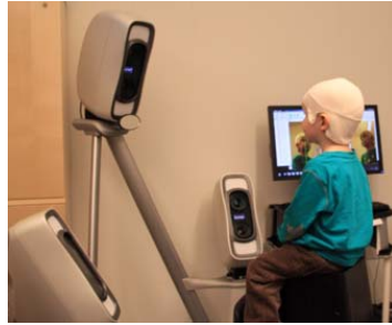
FIGURE 1: Canfield Vectra M3 scanner consisting of three pods each mounted with two Canon SLR Cameras.
