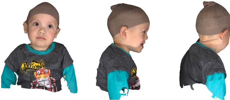
Figure 4.2: Three surface scans of a child, obtained during the same scan session. The figure shows the large shape variation that must be expected when scanning a young child. Take note of the mouth area and head position, for instance.
