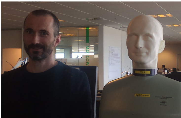
Figure 6.3: Test subject NH167 with the listener-specific head simulator based on subject NH167's head model.
