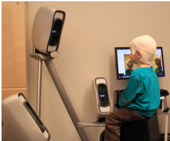
Figure 4.1: Scan setup with a Canfield scientific Vectra M3 surface scanner.
