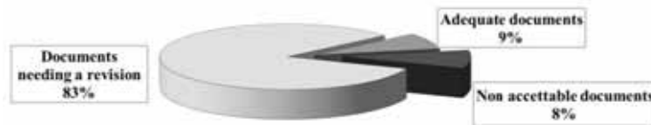
Figure 5 – Results from a statistical analysis on the congruence between the Safety and Health Plan and the Safety documentation drawn by the employers, in a number of real cases.
