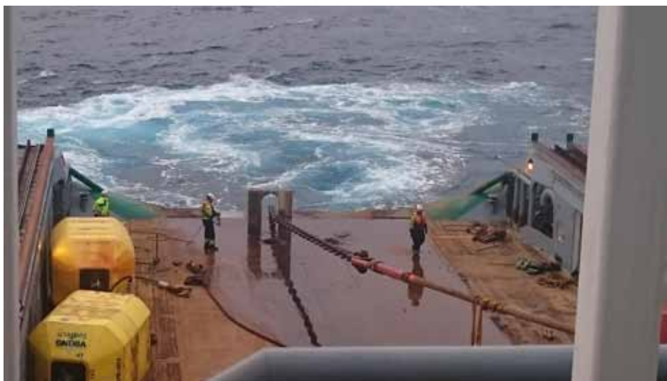
Figure 2 The sailors on deck have connected a chain. Seen from the bridge. As the winch starts to pull, the ship must be positioned correctly to balance the forces from the heavy load, weather and currents.
