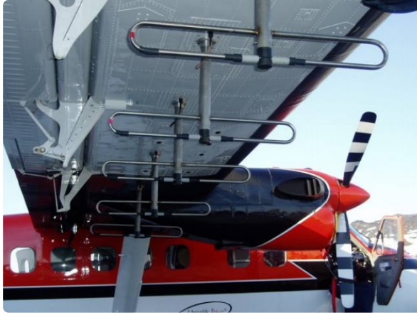
Figure 4.11: A photography showing the 5-element sub-array of folded dipole elements mounted under the right wing of the Twin-Otter aircraft.
