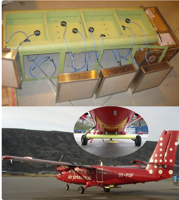
Figure 4.1: POLARIS 4-element antenna array: during assembly (top) and mounted under the fuselage of the DHC-6 Twin Otter aircraft (bottom).
