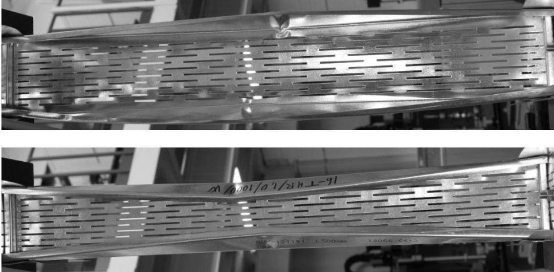
Fig. 7: Failure modes from test series 1-4. Test 8 - distortional opening (upper) and test 16 distortional closing (lower).
