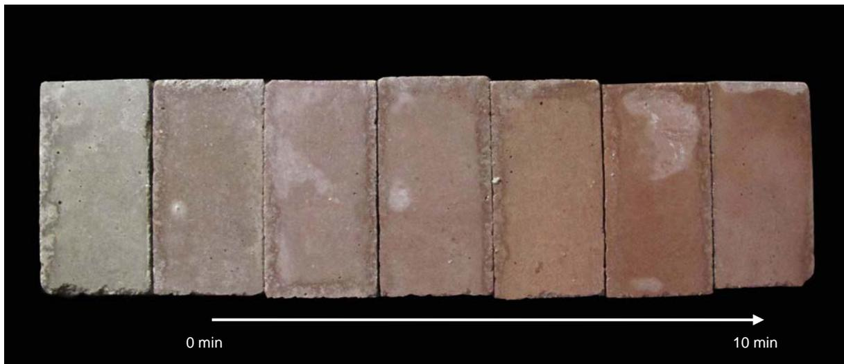
**Fig. 3.** Colour scale of moisturized mortar samples. The Grey colour of normal mortar gradually changes as the fineness of SSA particles increases. The first mortar sample to the left does not contain any SSA. The second sample contains un-treated SSA. Hereafter, the samples contain ground SSA of increasing fineness.
