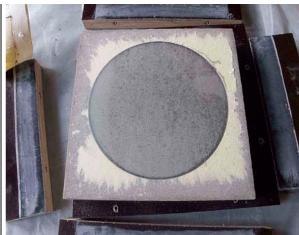
**Fig. 6.** Paper stuck to the hardened concrete tile.
