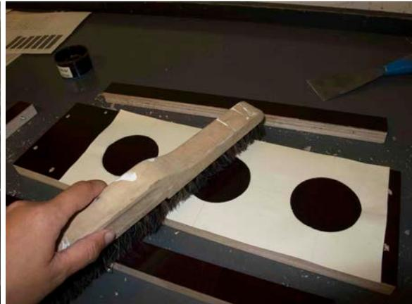
**Fig. 2.** The wet paper glued to the base.
