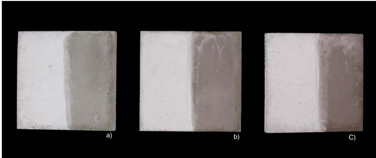
**Fig. 4.** a) sample –reference b) 10% cement replacement by un-treated SSA. C) 20% cement replacement by un-treated SSA. Half the tile was moistened .The Colour change was easier to see when the samples were wet.
