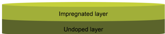
Figure 2. Principle sketch of two-layer pellet.
