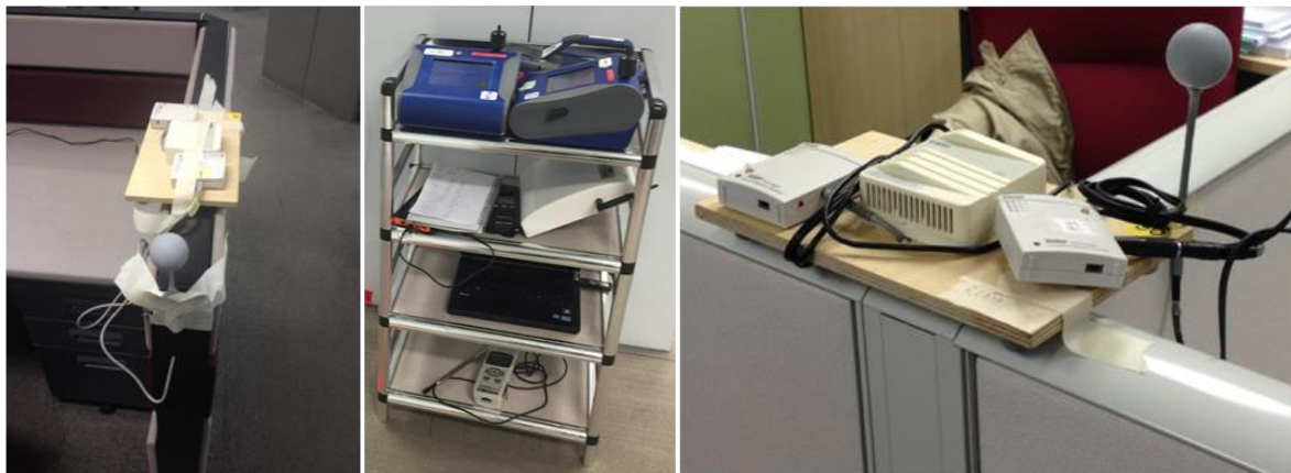
Figure 6-Data-logging equipment set-up and spot measuring equipment
