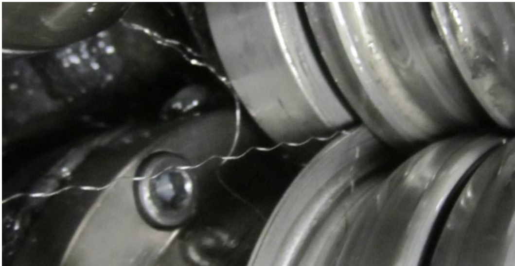
Figure 4-25: Edge swarf from tongue edge during winding
