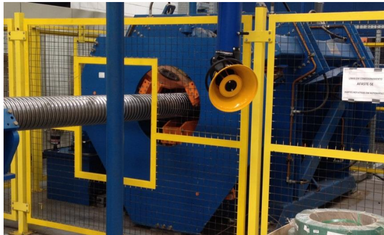
Figure 2-9: Caterpillar that constrains the carcass from rotating and transports the carcass from mandrel to the reel
