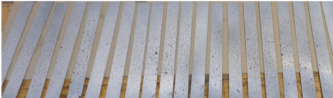
Figure 5-13: Tensile specimens with black on white speckle pattern for ARAMIS strain measurement
