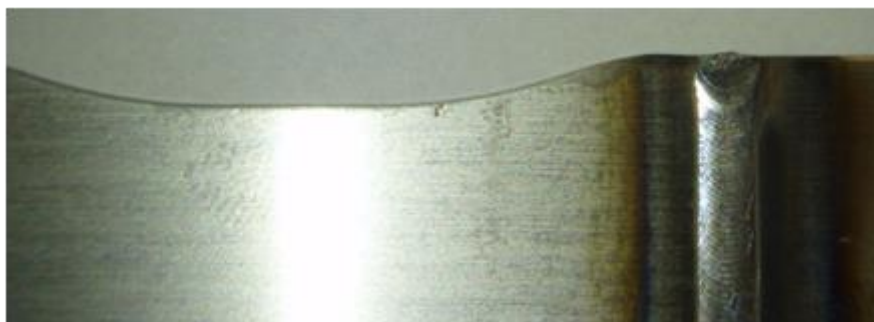
Figure 2-2: Weld and relief-cut on the left-hand-side of the weld
