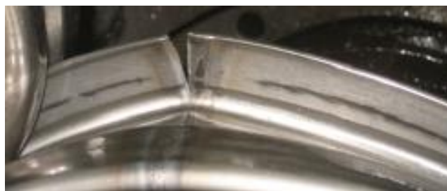
Figure 4-6: Weld fracture during winding
