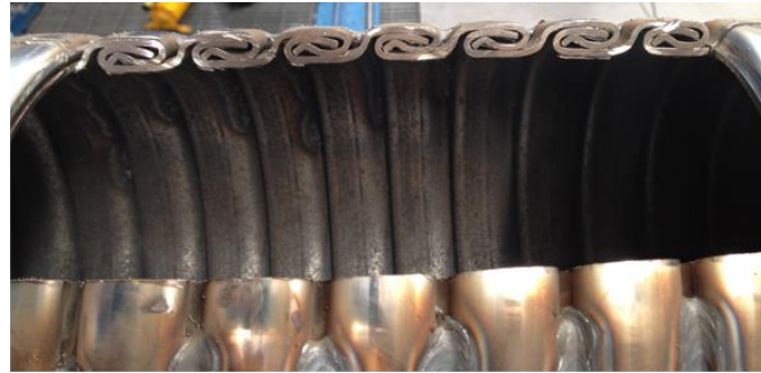
Figure 1-3: Typical measurement window being cut into carcass at production start and finish
