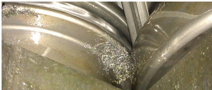
Figure 9-13: Edge swarf in roll forming caused by high normal pressure between tool curvature and workpiece
