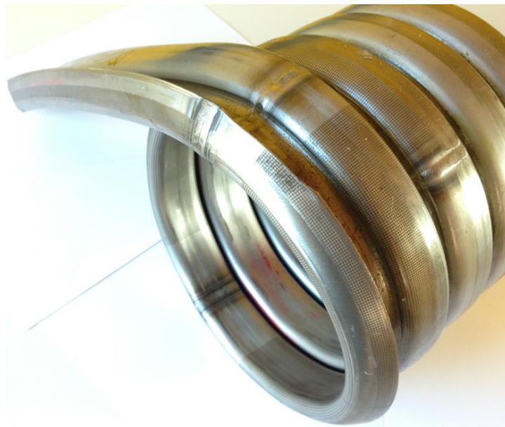
Figure 8-8: Typical carcass winding sample cut out of carcass for manual strain measurements with flexible rulers
