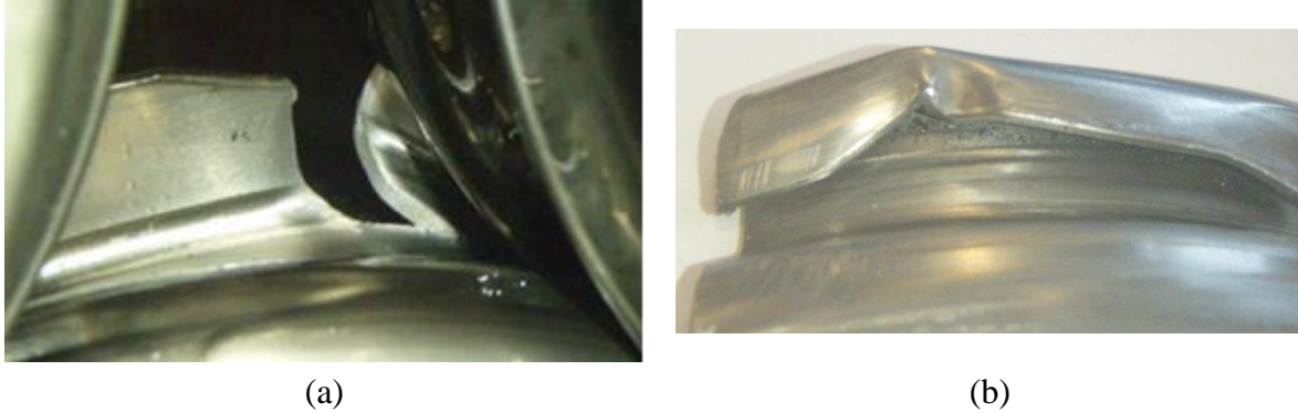
Figure 8-15: Weld relief-cut failure. (a) Fracture at bottom corner of the relief-cut between WT1 and WT2 during winding and (b) folding at weld relief zone due to interrupted bending of the tongue
