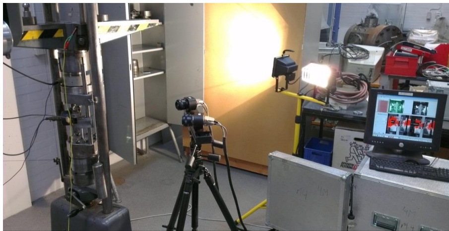
Figure 5-15: ARAMIS 4M system setup: light source, cameras, data acquisition box and computer
