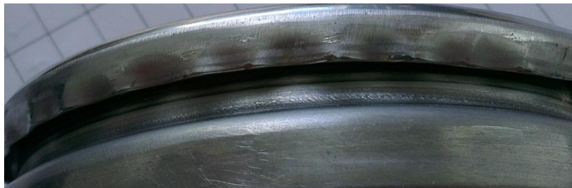
Figure 4-11: Tongue buckling after interlock
