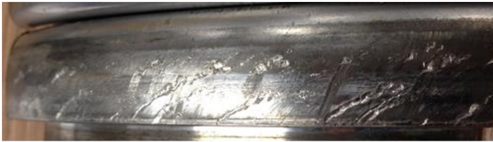
Figure 4-22: Severe scoring of the tongue as a result of bulge winding - only observable by cutting a window into the carcass.
