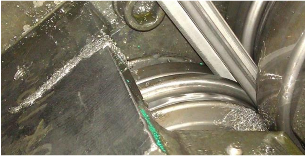
Figure 4-24: Edge swarf being dislodged in roll forming
