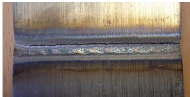
Figure 8-3: Fracture at transition from weld seam to HAZ during tensile testing correlating to weld fracture during carcass winding
