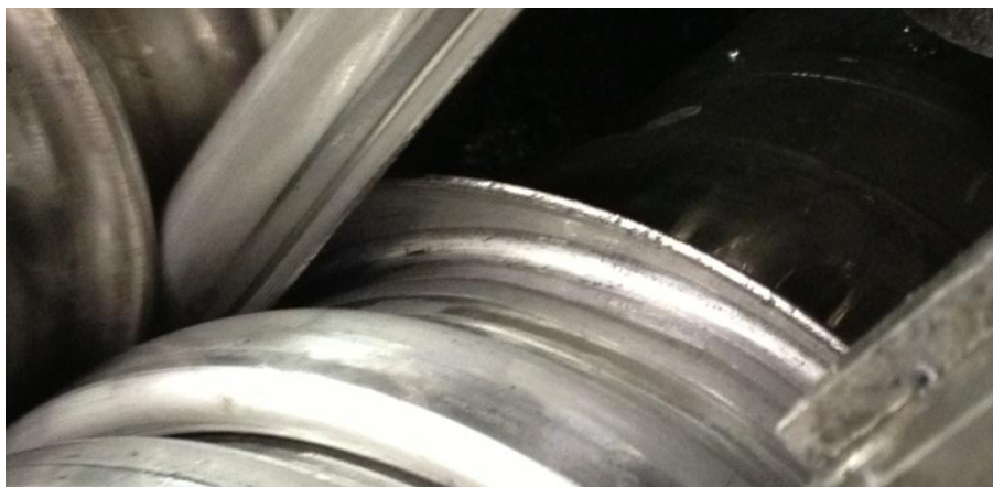
Figure 2-7: View of the interlock. There must be sufficient gap between the two legs of the profile to achieve a stable interlock – the gap is good in the shown picture
