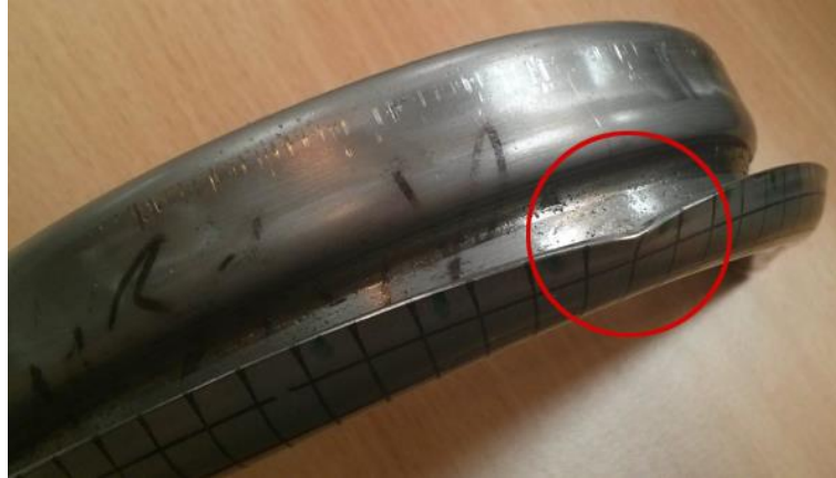
Figure 7-3: Position at which the bolt keeps the tongue in an upright position; it can be seen how the tongue closes away from the restraining bolt position resulting in lower strains away from there
