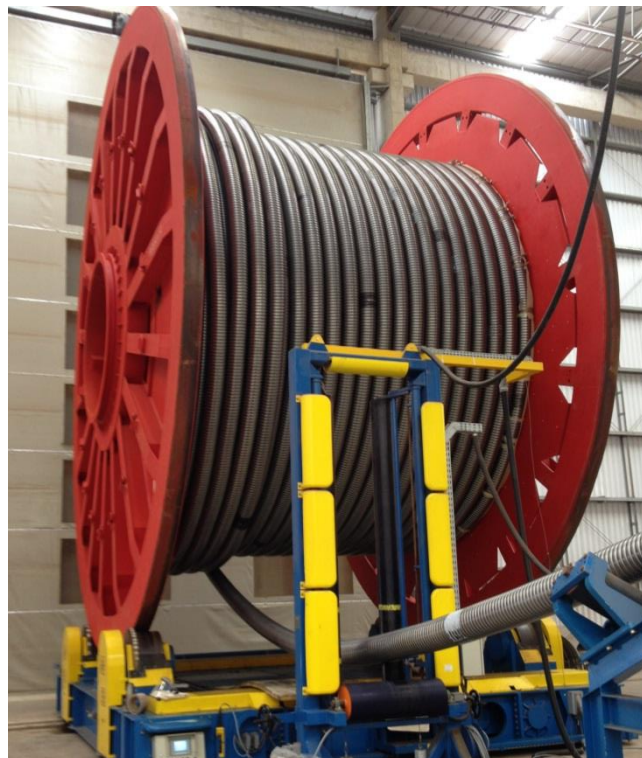
Figure 2-10: Reel with carcass. The radius of the reel flange is approximately 4m
