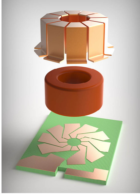
Fig. 2 Exploded view of the hybrid toroidal principle
