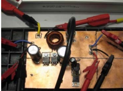
Fig. 5: The power stage and the output filter for the prototype.
