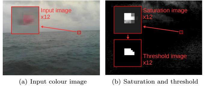
Fig. 7. Images from the obstacle detection algorithm.
