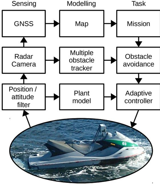
Fig. 1. System architecture - NASREM model.
