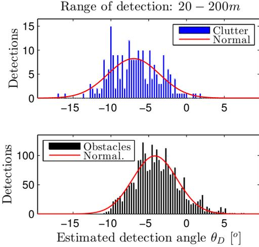
Fig. 9. Detection segmentation histogram from estimated height  $\theta(D)$ .
