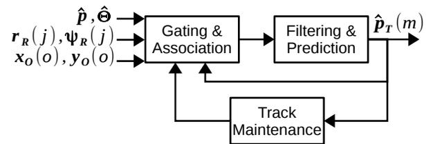
Fig. 8. Block diagram of the multiple obstacle tracker.
