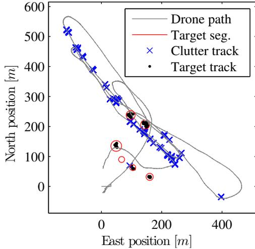
Fig. 11. Map of confirmed obstacles: tracks initiated and updated using radar only.
