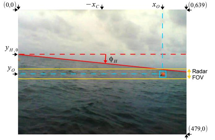
Fig. 4. Radar vertical FOV and the camera FOV.
