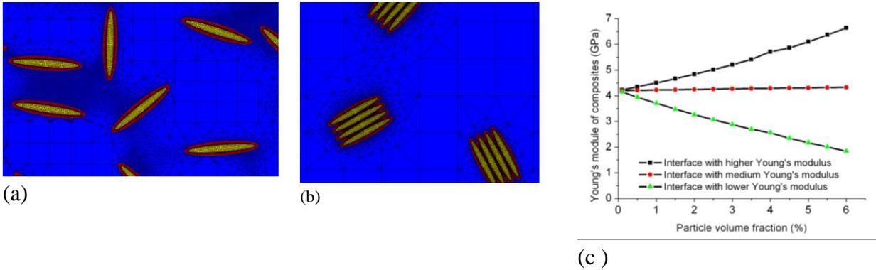
Figure 4. Generalized equivalent interface (GEIF) model for the analysis of nanoparticles in polymers (a, b) Finite element models with GEIF for exfoliated and intercalated (clustered) structures of nanocomposites, and (c) Effect of GIF properties on the properties of nanocomposite. Reprinted from [41, 42]\*.
