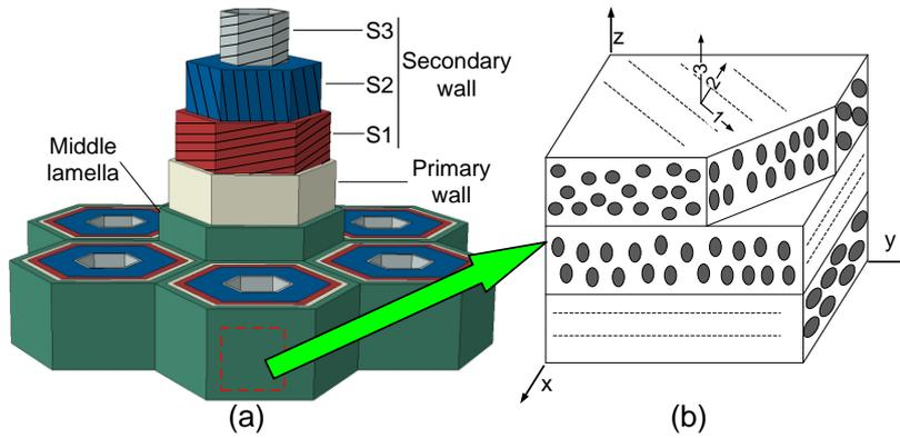
Figure 2. Multiscale model of wood as layered, cellular (a) and fibril reinforced (b) material [24, 25] \*. The thin layers S1, S3 with fibrils perpendicular to the fibrils in thick S2 layer control the buckling and fracture resistance
