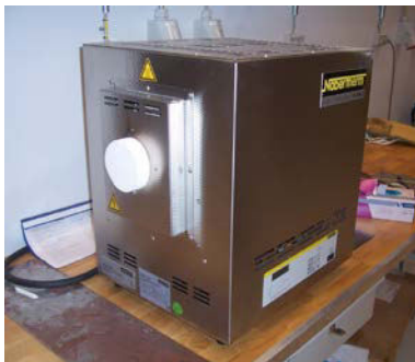
Fig. 12. a) Tube furnace Nabertherm RHTC 80-230/15 used for annealing of tungsten samples. b) Setting of the encapsulated tungsten samples in quartz ampoules during annealing inside the tube furnace.
