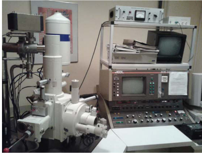
Fig. 18. One of the SEMs with an EBSD detector used for the EBSD analysis of this work: a JEOL JSM-840 with a phosphor screen as detector using CROMATIC v.2.10 software to index the measured bands (at DTU Risø campus).
