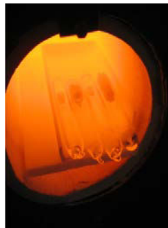
Fig. 12. a) Tube furnace Nabertherm RHTC 80-230/15 used for annealing of tungsten samples. b) Setting of the encapsulated tungsten samples in quartz ampoules during annealing inside the tube furnace.
