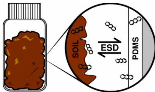
Drawing of equilibrium sampling device (ESD) for determination of thermodynamic activity by partitioning to micrometer thin polydimethylsiloxane (PDMS).
