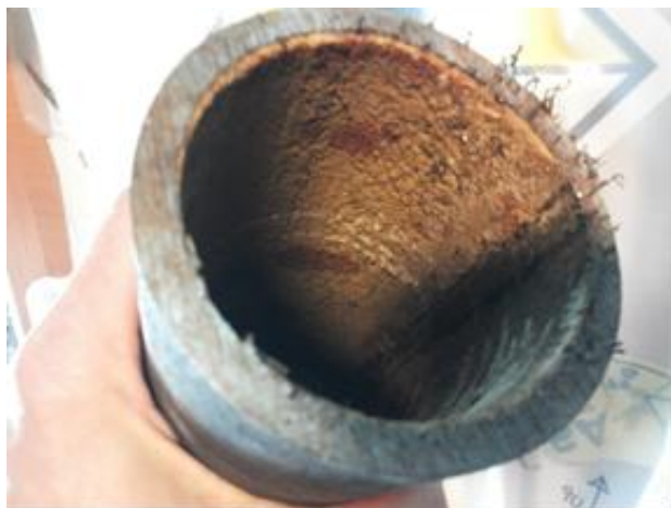
Figure 3. Visual appearance of the interior of a non-cleaned tube. The scale-thickness of the tube (tube No 7) was approximately 1mm.
