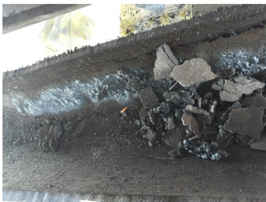
Figure 3. Visual appearance of the interior of a non-cleaned tube. The scale-thickness of the tube (tube No 7) was approximately 1mm.
