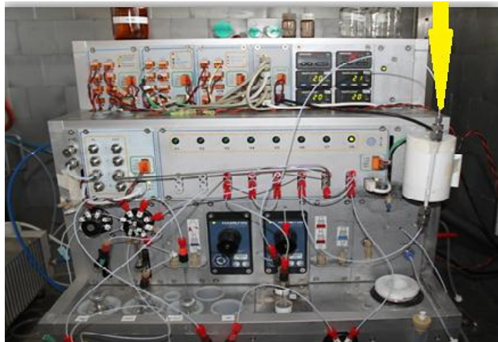
Figure 5-5. The radiofluorination apparatus with the column placed outside the column oven (yellow arrow)
