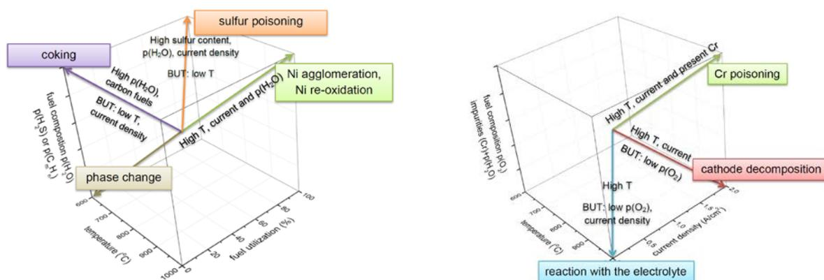
Fig. 1 Dependency of anode and cathode degradation mechanisms (examples) on operating parameters.
