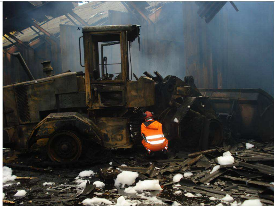
Figure 5 Examination of the wheel loader revealed that the universal (cardan) joint and shaft was missing. Windows in the driver's cabin melted in the intense heat. Tires are burned away. Source: Police investigation, photo in useful quality kindly provided by an official from The Danish Working Environment Authority.
