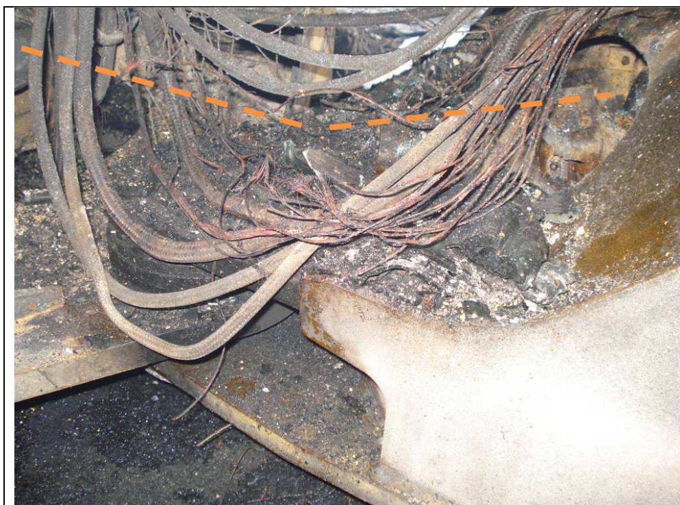
Figure 6 Torn electrical cables and fire damaged hydraulic hoses. Dotted line shows approximate position of missing universal (cardan) joint shaft. Hydraulic hoses appear intact. Source: Police investigation, photo in useful quality kindly provided by an official from The Danish Working Environment Authority
